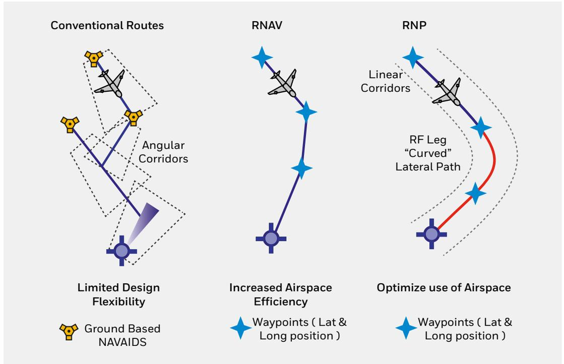
Figure 1: Conventional Navigation versus RNAV and RNP
