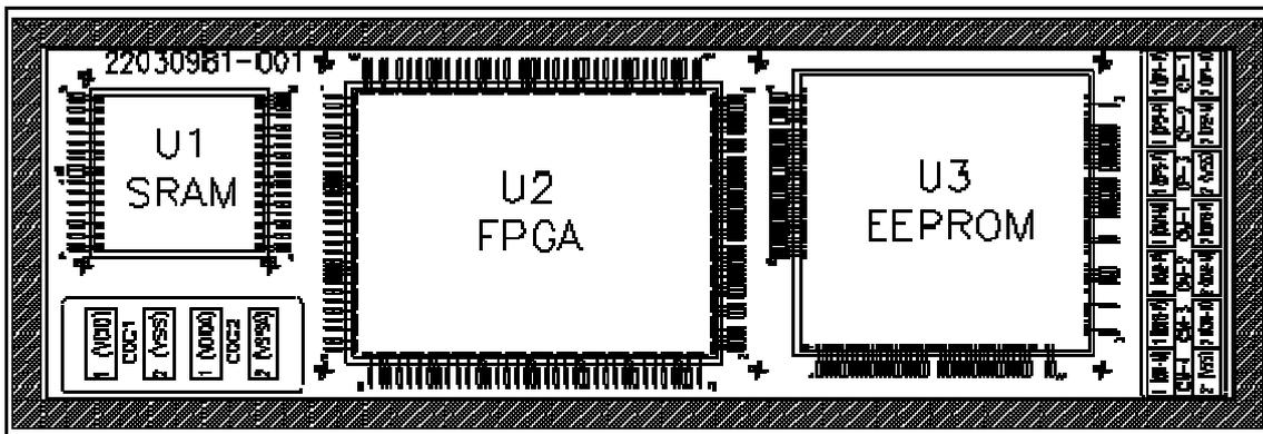
**FIGURE 6: RPDA Package Component Floorplan, Top View.**
