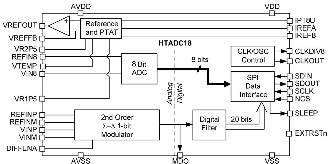
**FIGURE 1: Deep Trek High-Resolution A-to-D (HTADC18) Block Diagram**
