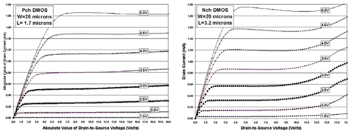
Figure 3: Extended Drain (DMOS) I-V Characteristics
