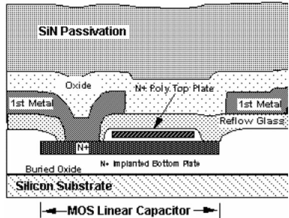
Figure 2: Capacitor Structure
