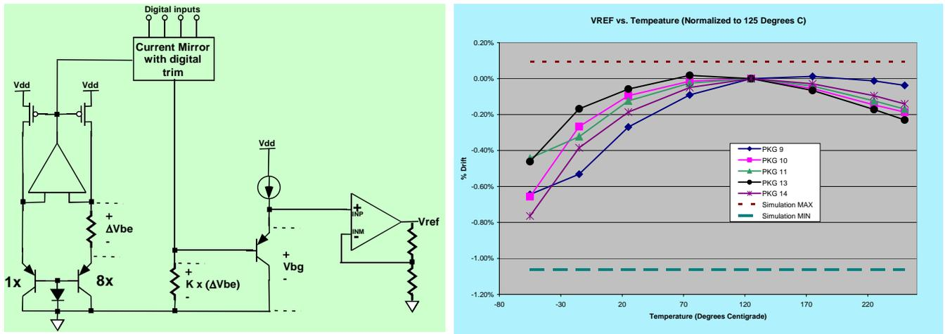
**Figure 4 : Bandgap Voltage Reference Using Lateral PNP Transistors**
