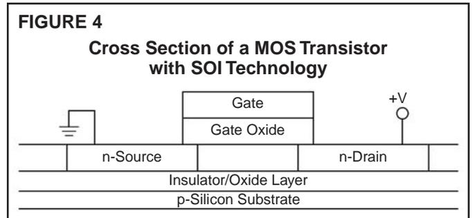
layer, as shown in Figure 4. SOI limits appear to be 300 degrees C, the point at which junction leakage currents become theoretically prohibitive, but there have been reports of success with operations as hot as 400 degrees C.
