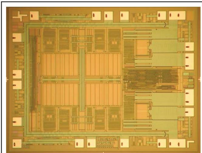
**NETL-funded tests of the op amp by Sandia National Laboratories have demonstrated that high temperature silicon on insulator technology can perform well at temperatures higher than 300 degrees C. After more than 1,000 hours at 300 degrees C, the tests show a maximum of only 20 $\mu$ V offset voltage.**
