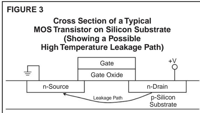
istor is an electronic switch that consists of three basic elements: the source, the gate, and the drain. Figure 3 is a simplified sketch of a MOS transistor.
