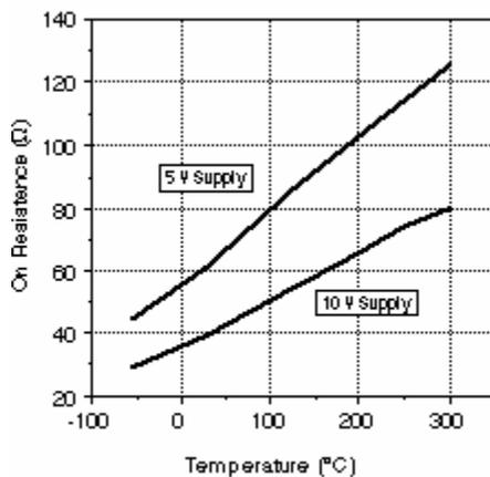
Figure 5. Quad Analog Switch "ON" Resistance vs. Temperature
