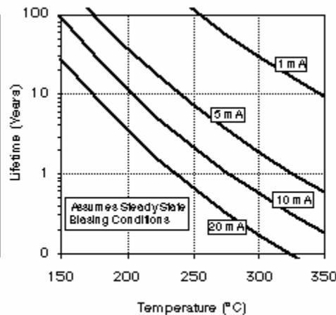
Figure 6. Quad Analog Switch Lifetime vs. Temperature
