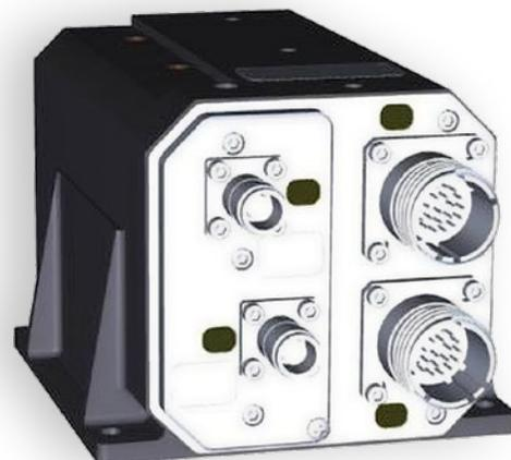
A revolutionary concept that will not only produce a modern, state-of-the-art altimeter, but will also facilitate voice of the customer needs identified previously. Honeywell is utilizing the Radar Altimeter Common Core (RACC) as the main building block and packaging it into a Radar Altimeter that is form fit and enhanced function replacement for all APN-209 standard configurations.
