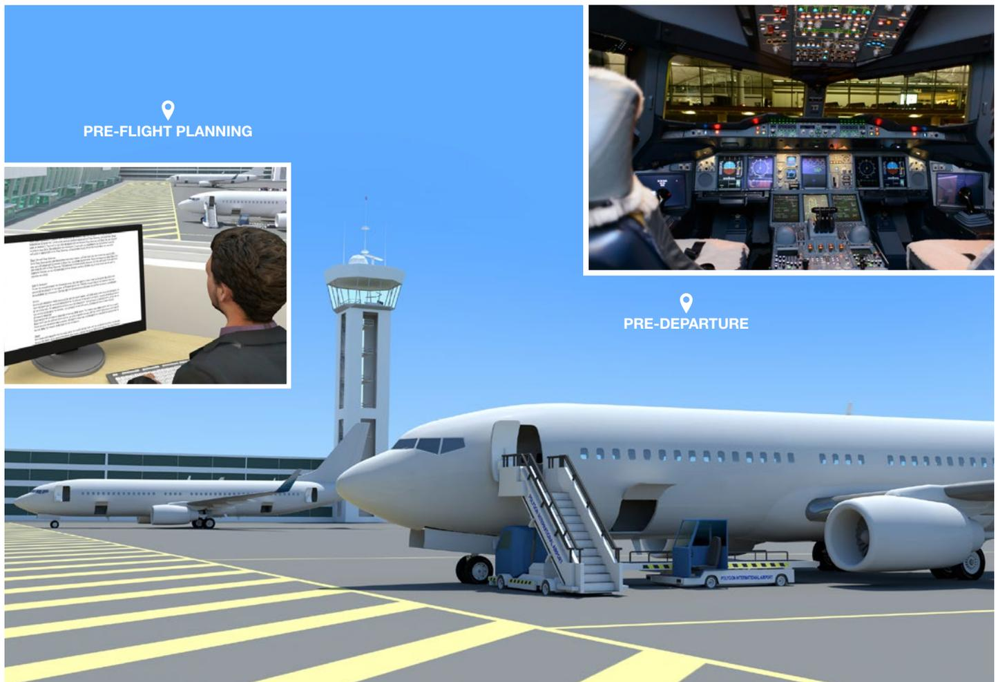
Honeywell's FMS Datalink Service allows the flight crew to quickly and efficiently uplink the flight plan and latest wind and temperature information to the FMS via datalink. The service saves time over manual entry, reduces the risk of data entry errors, and assures the FMS has the most up-to-date information to ensure optimized flight level recommendations.
