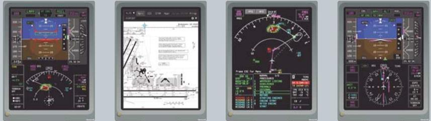
Five, DU-1080 LCD configuration: Full flight deck integration featuring two PFDs, two MFDs, and engine instruments (Available on L-382G)
