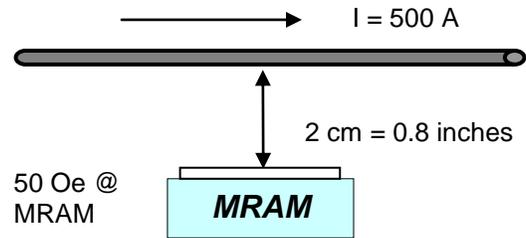
Tabulated below, based on Equation 6 for the given current, are minimum separations, in four distance units, between the surface of the cylindrical wire and the surface of the MRAM, that result in attenuation to 50 Oe of the SMF from the current in the wire:
