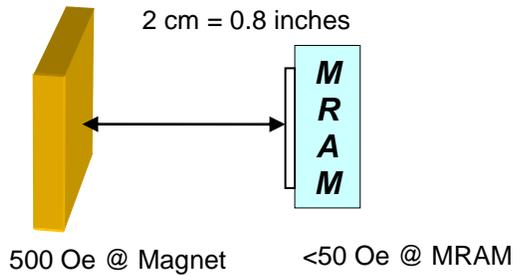
**Example 2:** A cylindrical permanent magnet with a diameter of 0.5 cm, thickness of 0.2 cm, and a surface magnetic field of 2,500 Oe, produces, at a distance of 2 cm, a magnetic field of 10 Oe, which is well below the protection threshold of the MRAM. The SMF value for this case is attenuated by more than a factor of 250 in a distance less than one inch.
