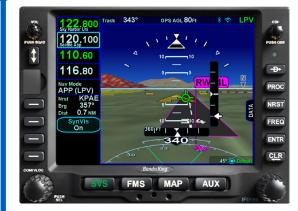
The AeroNav 910 is the flagship of the AeroNav product line. It gives the pilot the optimal situational awareness using both out-the-window and in-trail 3-D synthetic vision, internal ADAHRS and wireless connectivity.
