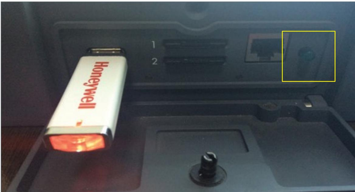
**NOTE:** During the load process, both lights will flash amber. When both the lights turn green; it indicates that the configuration loading is successful. If the left light flashes and the right light is steady amber, it indicated that the configuration has failed. The ADG100 will write a status file to the USB with the file name `install_tailnumber.log`.
