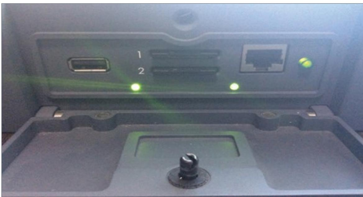
Cycle power to the ADG100 once configuration file load is complete. It can take up to one minute for ADG100 to complete self-test and activate Wi-Fi.
