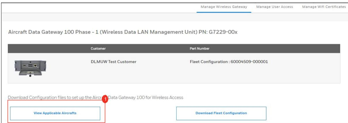
**NOTE:** You can reset the ADG100 to factory default by downloading the **dlmuwcfg\_reset.zip** file from the **Additional Actions** section on the **Manage Wireless Gateway** page. The process of loading the reset configuration file is the same as that of the **Uploading the Configuration File to ADG100**. However, loading the reset configuration file disables the wireless access on the ADG100.
