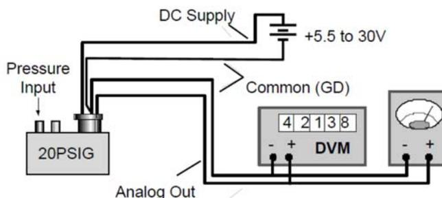
**Figure 4.6 — PPT Pressure to Analog Voltage**
