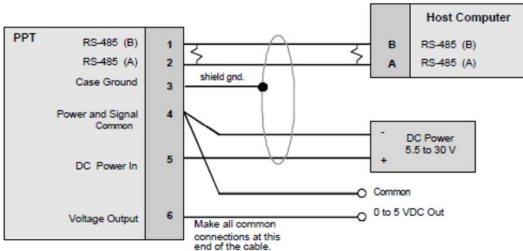
Figure 6.3 – Connection for RS-485 Operation and Analog Output
