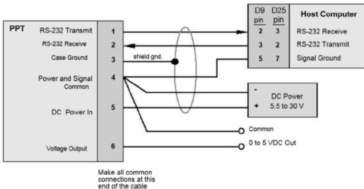
**Figure 6.2 – Connection for RS-232 Operation and Analog Output**
