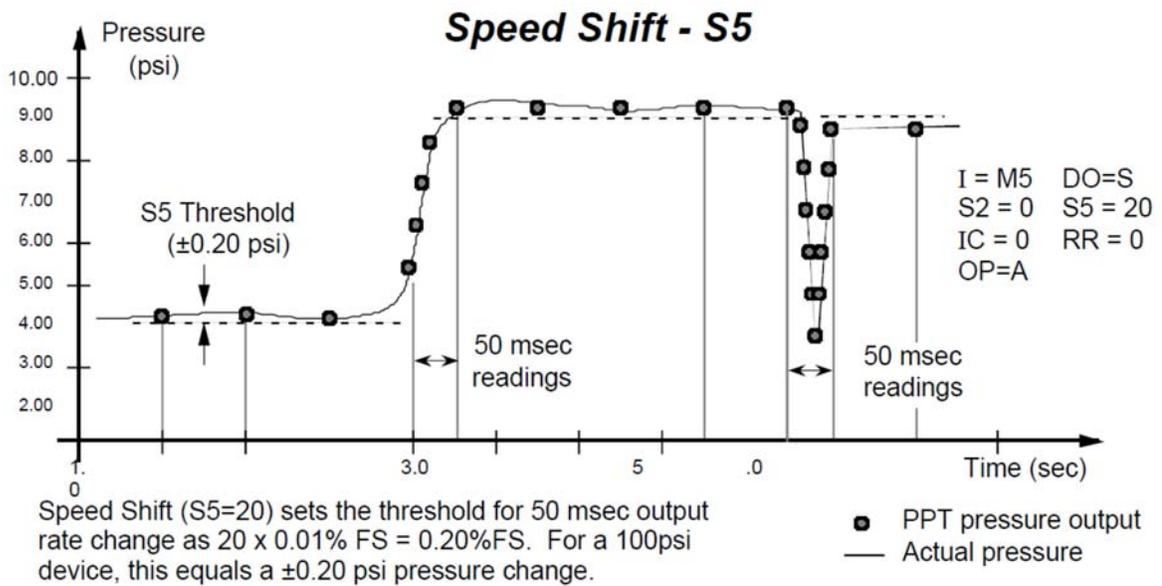
**Figure 4.12 – S5 Speed Shift Command Example**
