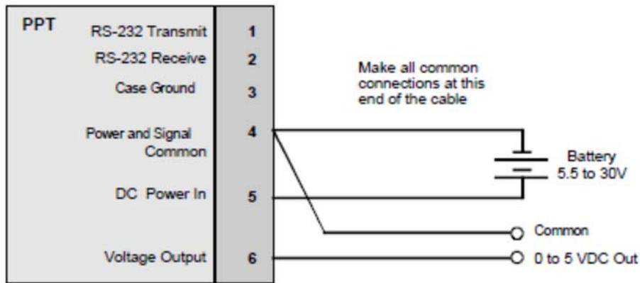
Figure 6.4 – Connection for Analog Output and Battery Operation
