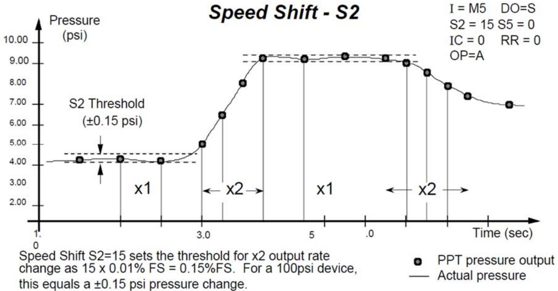
Figure 4.11 - S2 Speed Shift Command Example
