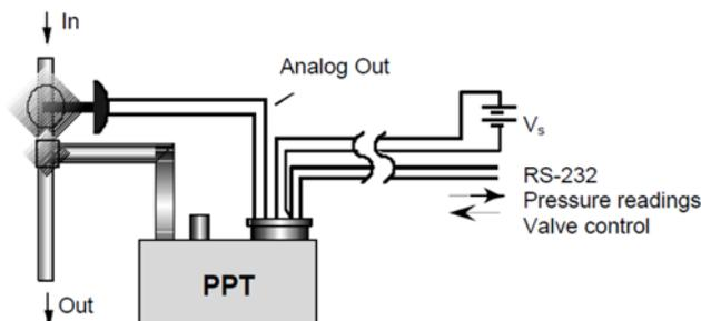
**Figure 4.7 — PPT Pressure Readings and Analog Voltage Control**
