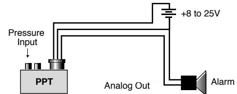
Figure 10. Pressure Limit Activated Alarm
