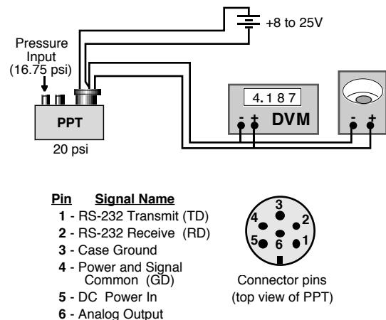
Figure 1. Connection for Analog Output Mode
