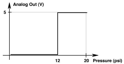
Figure 9. Pressure Trip Point Setting
