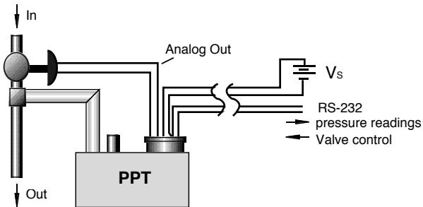
*Figure 12. Digital Pressure and Analog Valve Control*
