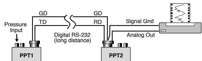
Figure 8. Sensing Remote Analog Pressure
