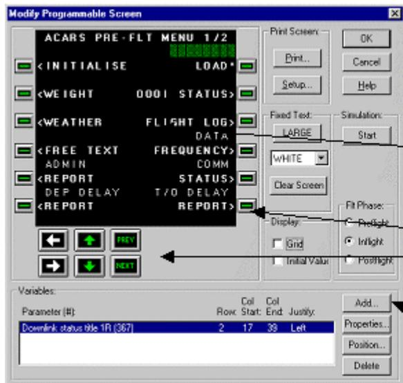
A picture of the selected MCDU screen, as well as the controls needed to edit the screen are provided in a single window.
