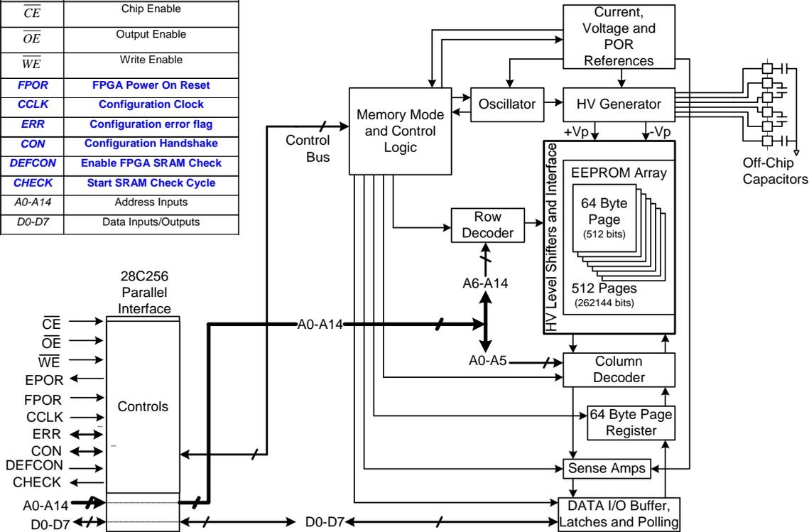
**FIGURE 4: HTEEPROM Parallel Interface Configuration**
