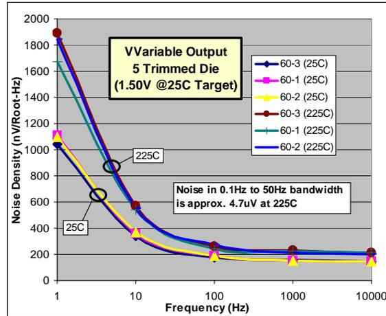
Figure 7: Buffered Reference Output Low-Frequency Noise Characteristics
