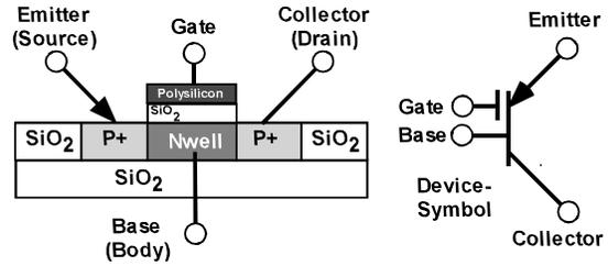
**Figure 2: Lateral PNP Structure and Device Symbol**
