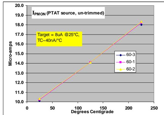
Figure 9: Temperature-scaled Current Source,  $I_{\text{temp2}}$  (PTAT) Output
