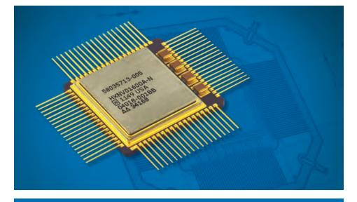
The Honeywell 16 Megabit radiation hardened low power non-volatile Magneto-Resistive Random Access Memory (MRAM) offers high performance and is designed for space and military applications. The part can be configured as either a 2,097,152 word x 8-bit or a 1,048,576 word x 16 bit MRAM through an external pin setting.
