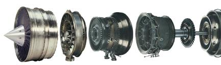
Fan Module Front Frame Module
