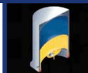
Ammonia Tank and Accumulator
