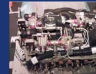
Carbon Dioxide Removal Assembly (CDRA)
