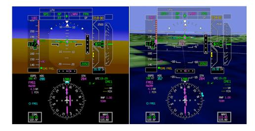
In addition to SVS, enablement of this option also enables the Integrated Navigation (INAV) functionality for the MFD moving map display. As shown in the figure below, the INAV functionality enhances the crew's navigational situational awareness through depictions of the lateral flight plan enhanced with a moving map, and vertically via the Vertical Situation Display (VSD) and provides new options for the crew to interact and view the flight plan graphically vs textually:
