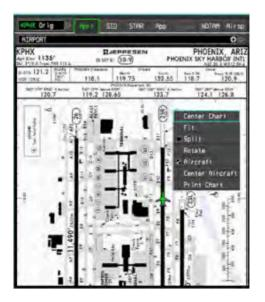
With E-Charts and Maps Enabled, Airport Diagrams and other Charts can be displayed in the crew's forward field of view, with a continuously updating own ship position shown on the chart.
