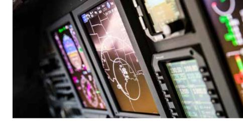
Wing Aviation's maintenance team is also happy with the new flight management system and its impact on departure reliability. Van Winkle was already having problems with the old CRT screens, and loves the new LCD displays because they're a lot lighter and don't require a complex cooling system. "Just like our approved Electronic Flight Bag system, the new displays help reduce weight, gain efficiency, and improve fuel burn," she says.
