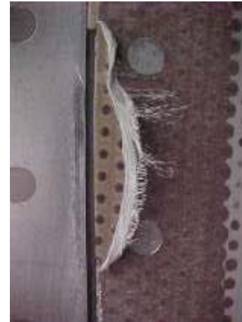
Inlet Screen Peeling at Leading Edge
