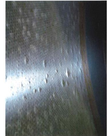
Inlet Barrel Blistering
