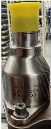
Post SB AS907-73-9003 P/N 2718964 Hydra-Electric
