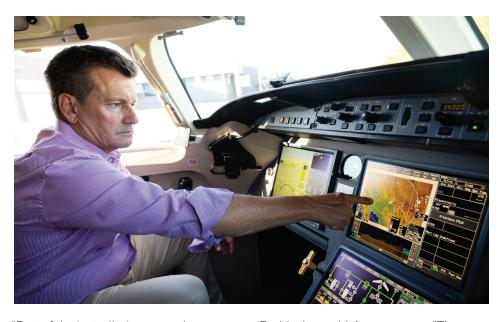
"Part of the instrallation upgrade invovled replacing the data loader unit," explains Adam DeRosa, Director of Maintenance at VCAP Aviation. "The new DLMU greatly increases the speed of data loads. Basically every other week we're doing a database update here at the hangar, and the new data loader really streamlines the process."
