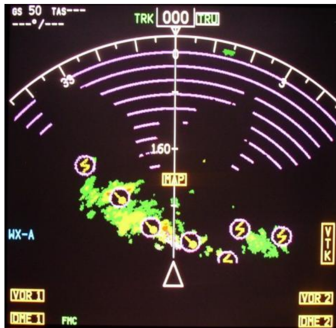
Figure 5. Radar Images of Weather Cells showing REACT, Predicted Lightning, and Hail Icons
