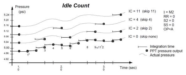
Figure 4.15 – Idle Count (IC) Command Examples
