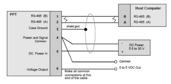
Figure 6.3 – Connection for RS-485 Operation and Analog Output
