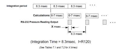
Figure 7.5 – Timing Diagram for 120 Readings per Second
