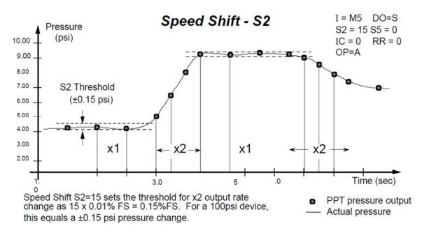
Figure 4.11 – S2 Speed Shift Command Example
