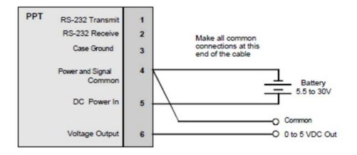
Figure 6.4 – Connection for Analog Output and Battery Operation
