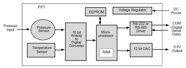
Figure 4.1 – PPT Block Diagram
