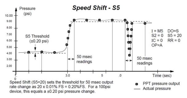
Figure 4.12 – S5 Speed Shift Command Example
