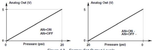
Figure 4.3 – Factory Set Output Levels
