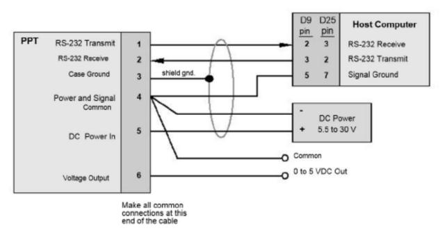
Figure 6.2 – Connection for RS-232 Operation and Analog Output
