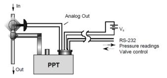
Figure 4.7 — PPT Pressure Readings and Analog Voltage Control
