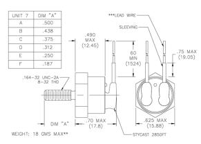
Typical Dimension for all configurations. \*\* "WEIGHT" does not include weight of lead wires. \*\*\* Wire (where applicable) MIL-W-22759/43 712
