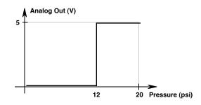
Figure 9. Pressure Trip Point Setting
