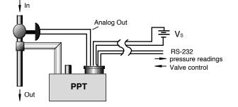
Figure 12. Digital Pressure and Analog Valve Control
