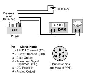
Figure 1. Connection for Analog Output Mode
