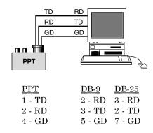
Figure 3. Connections for Digital Command Mode
