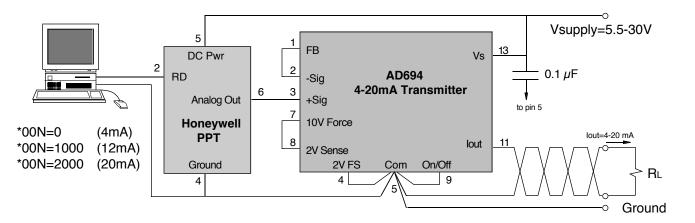
Figure 2 - Computer control of 4-20 mA current loop
