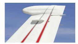
The AMT-700 is typically housed under a tail-mounted radome, but can also be mounted at several locations on the fuselage
