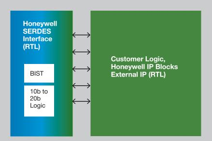
Both 4 lane and 8 lanes HX5000 SERDES macrocells can be instantiated with to create systems with 32 – 40 lanes (power dissipation can become a limiting factor). The interface to the core logic includes specialized high speed parallel interface logic and Built in Self-Test (BIST) logic.
