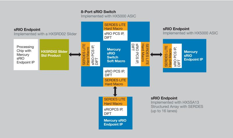
Multiport Switches and Endpoints are common in communication network applications and a more direct "transmitter to receiver" configuration is used for applications like image sensors data processing.
