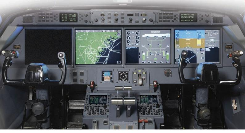
Honeywell's original DU-1310 Cockpit displays (p/n 7028140-901/-905) can no longer be repaired.
