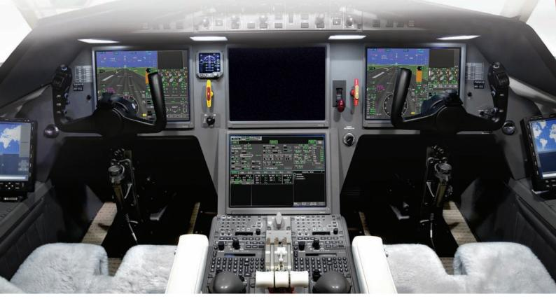
Honeywell's original DU-1310 Dassault EASy Cockpit displays (p/n 7028140-901/-905) can no longer be repaired. If your aircraft is equipped with the legacy DU-1310 displays we encourage you to sign up for our HAPP DU-1310 Extended Coverage. Once covered should you experience a display failure, Honeywell will cover the cost for the replacement of both displays with newer units.
