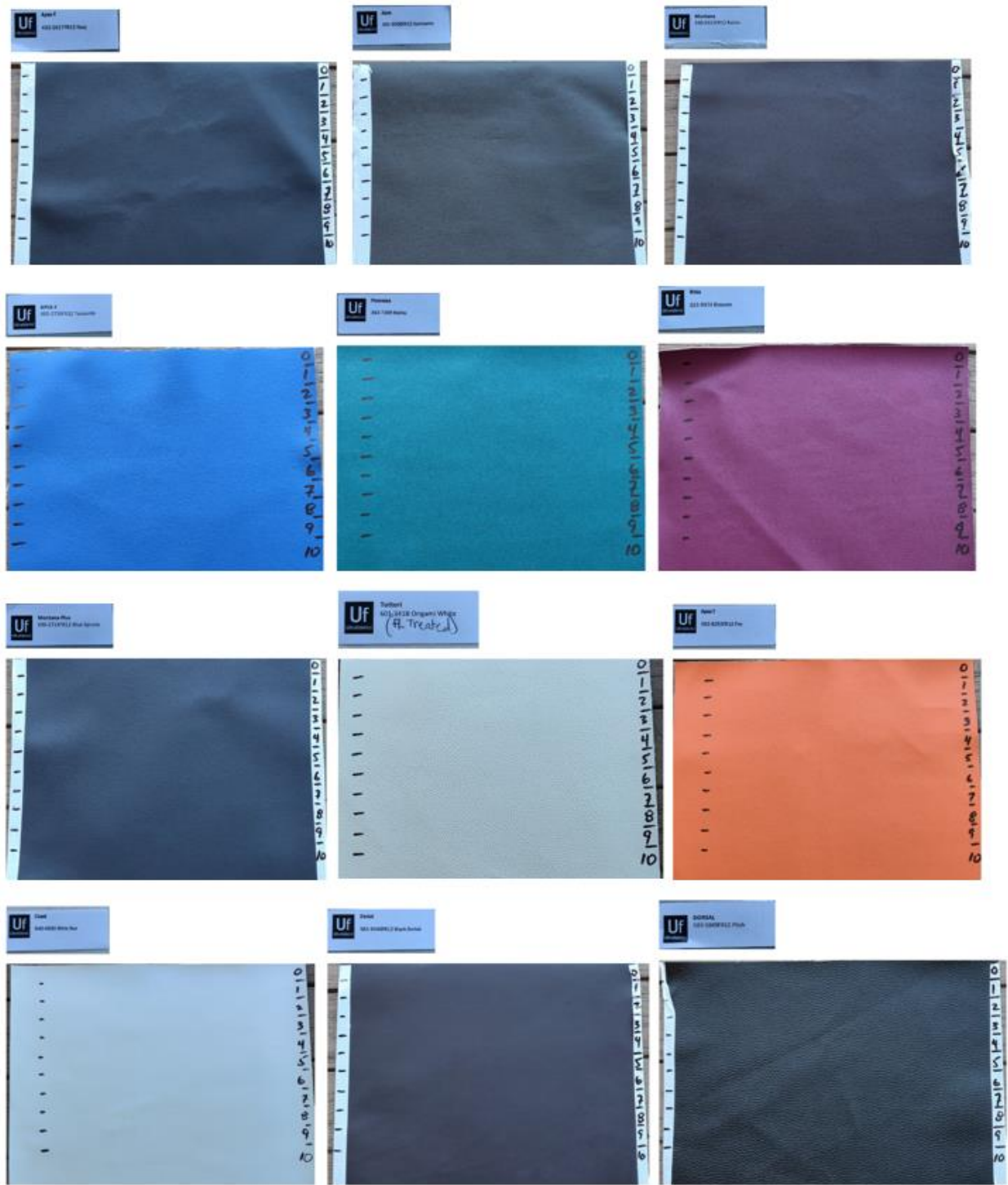
Figure 33. Ultrafabrics Samples, Progressive Exposure to 40 J/cm 2
