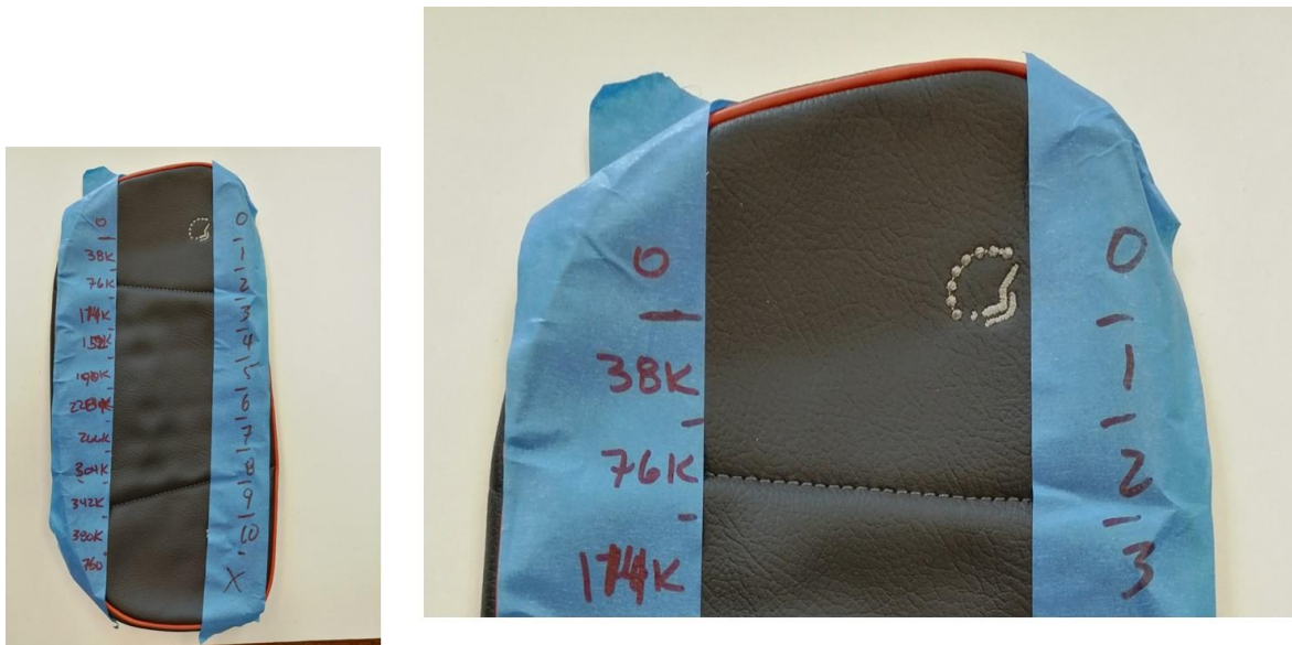
Figure 29: Leather armrest after progressive UV-C exposure. Photo on right is close up of the upper portion of the left photo, with UV-C dose marked.
