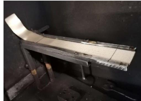
Figure 37. Seat Belt Flame Resistance, Test Set-up
